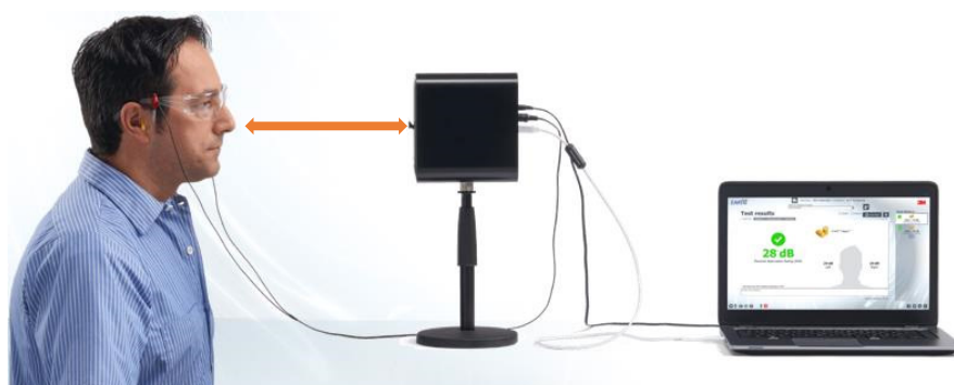
Figure 4. The distance from the testee’s nose to the clip on the loudspeaker was 40 cm.
